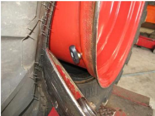
3. Insert the AGRI TPMS sensors in the correct numerical order.
