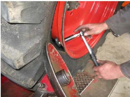
5. Tighten down to 5 ~ 8Nm.
