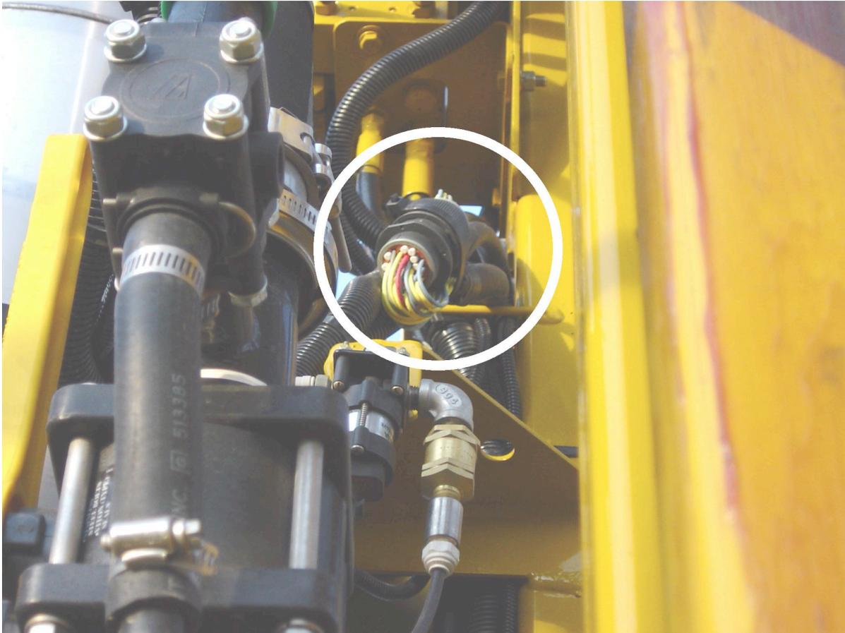
2. Disconnect the wiring harness and plug the SprayTest adapter harness in between.
