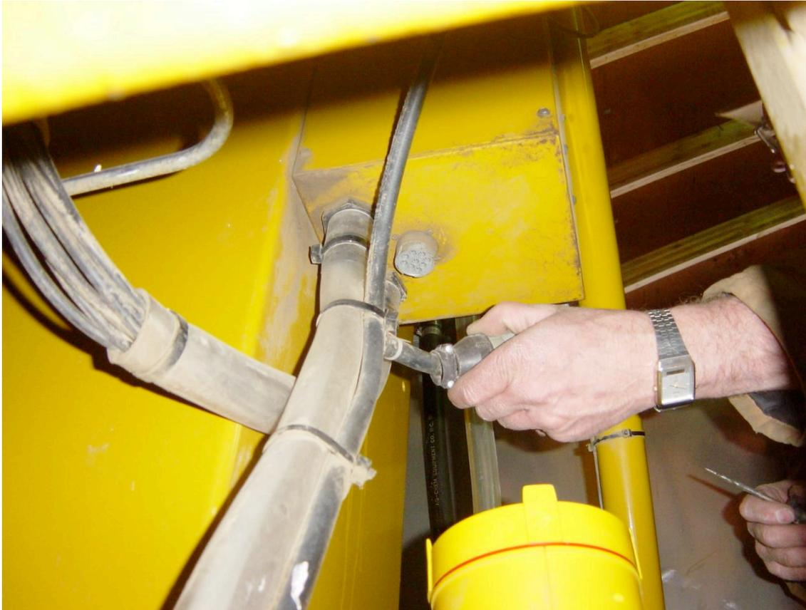
2. Disconnect the wiring harness from the bottom of the valve box and plug the harness into the plug on the valve.
