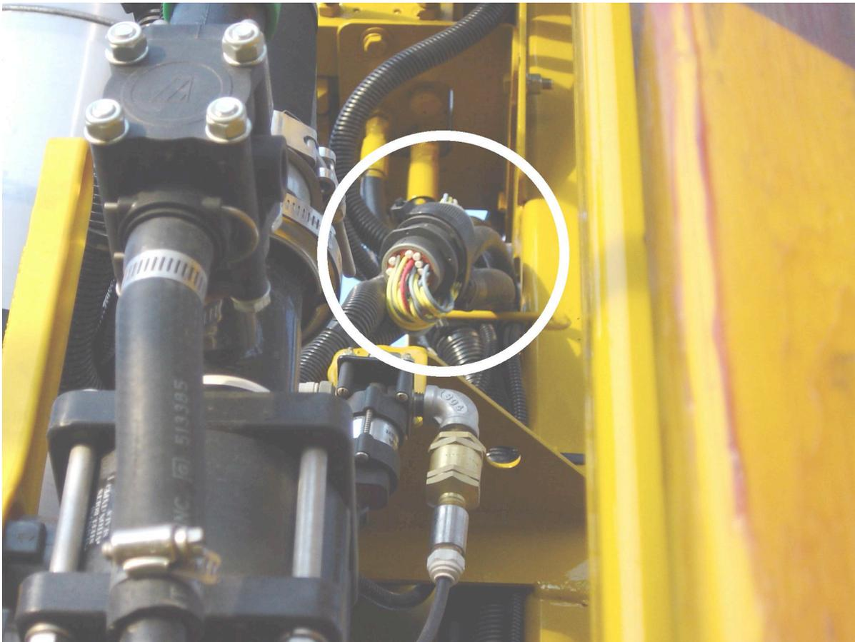
4. Disconnect the wiring harness and plug the SprayTest adapter harness in between.
