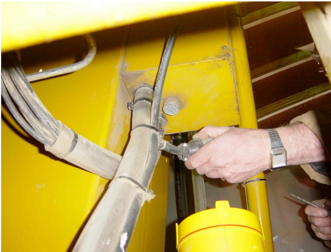
4. Disconnect the wiring harness from the bottom of the valve box and plug the harness into the plug on the valve.
